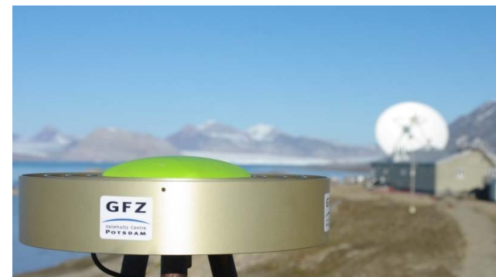
GRUAN polar GNSS station
